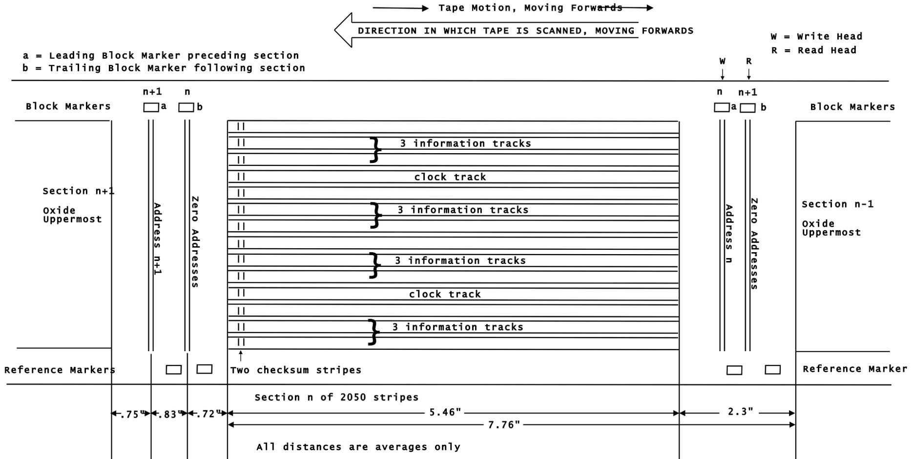
When moving forwards the tape moves from left to right, and is therefore scanned from right to left
