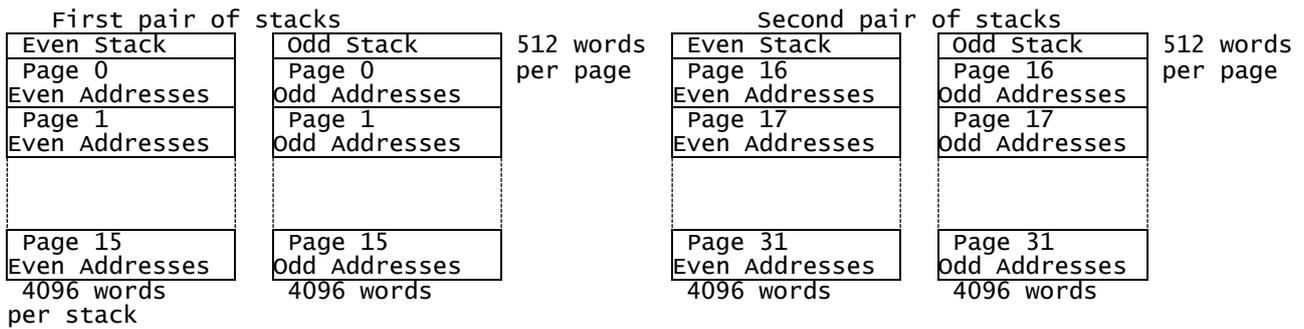
When obeying a programme instructions are taken from the core store in pairs. A pair of instructions consists of an instruction from an even stack plus the next instruction from the odd stack in the same pair. Provision is made in the machine for the cases
