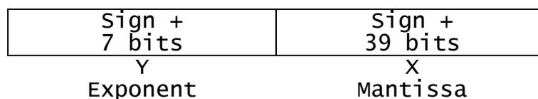
True complements are used for negative number so that when a non-zero number is in standardised form
