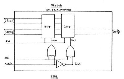
The new building block  $2K_BY4_MEMORY$  is defined from two 2114 1K X 4-bit memory chips and the logic circuitry necessary to select one chip or the
