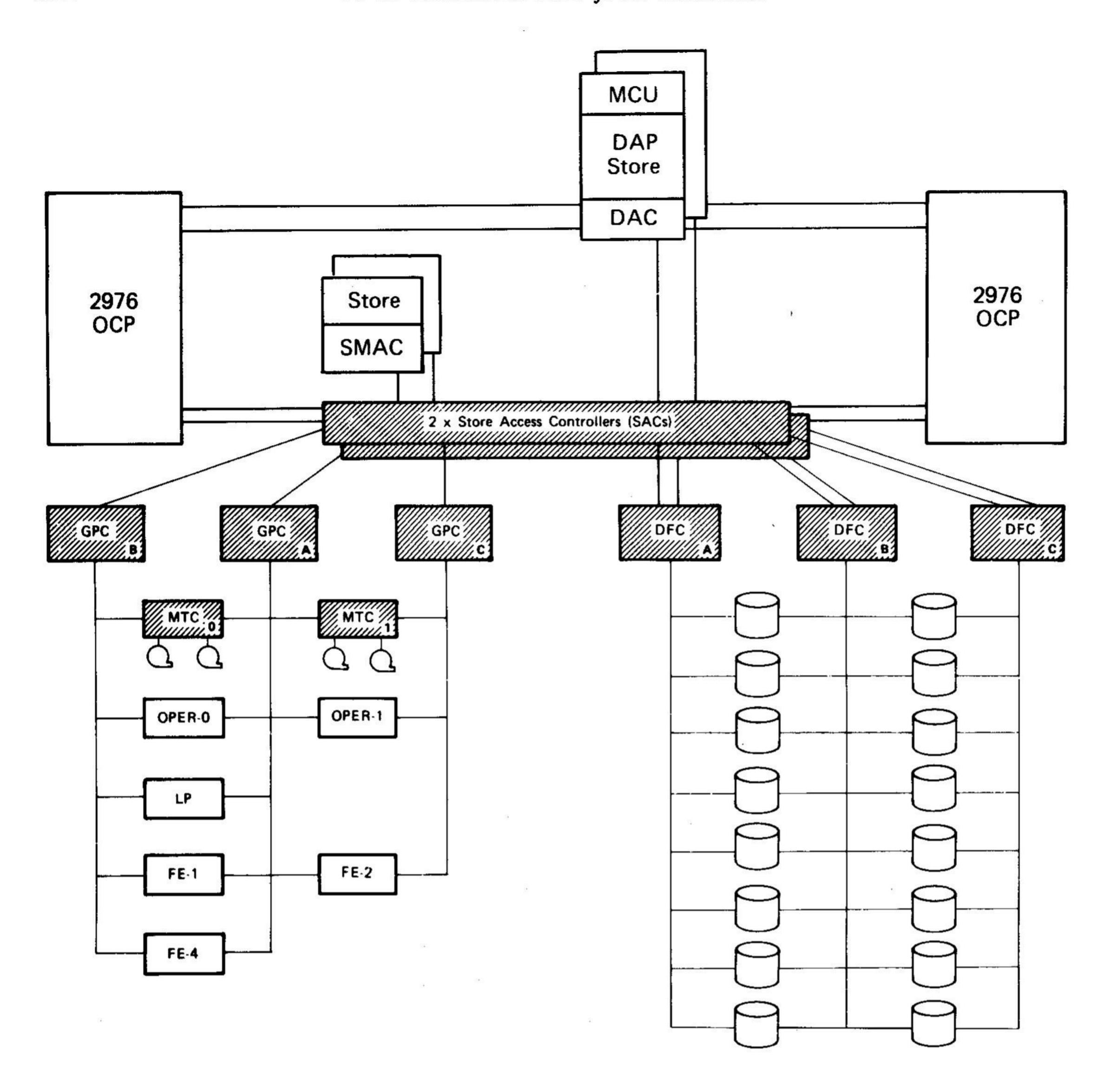
Key: Order Code Processor GPC - General Peripheral Controller DAP - Distributed Array Processor MTC - Magnetic Tape Controller DAC - DAP Access Controller OPER - Operator Console MCU — Master Control Unit Line Printer SAC - Store Access Controller FE Front End SMAC – Store Multiple Access Controller (Communications Processor) DFC - Disc File Controller Mbyte - 1,048,576 bytes
