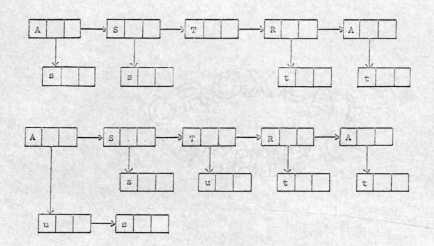
This system of lists with three-field cells was chosen as the basis of the lists used in ASTRA.
