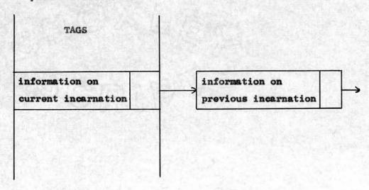
When a name is redeclared, a cell is taken from an Available Space List and the old TAGS information copied into it. The information relating to the new declaration is placed in the TAGS array together with a link to the pushed-down cell. The same type of cell and list processing scheme is used in a number of contexts throughout the compiler, some of which will be mentioned later.
