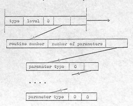
A list processing scheme which packs the information closely, as this does, leads to slightly reduced speed of operation because of the amount of unpacking to be done, but has the essential advantage of minimising the total amount of storage used, which was at a premium on KDF9.
