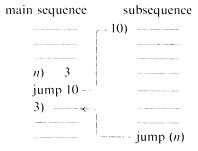
In the same way the instruction n) m makes a jump n instruction transfer control to one of several different points depending on the computed value of m. This device is known as a multi-way switch.
