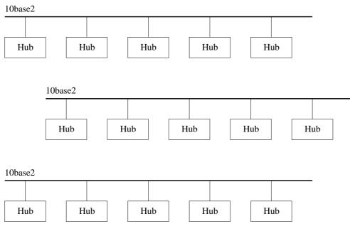
Figure 4: Hubs connected by 10base2
