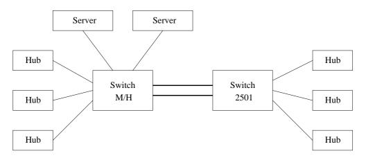
Figure 5: Hubs interconnected using switches
