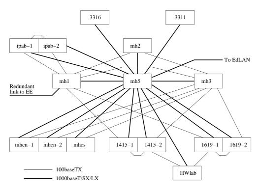
Figure 6: JCMB network using switches throughout
