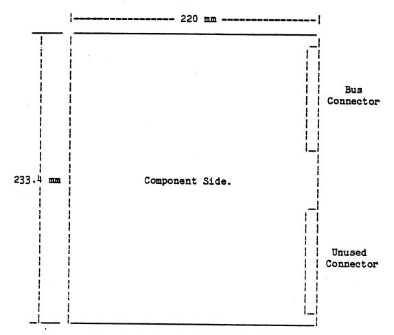
The unused connector position may be used freely to provide off-board or inter-board connections. It is intended that this facility should be used to communicate with other buses and systems.
