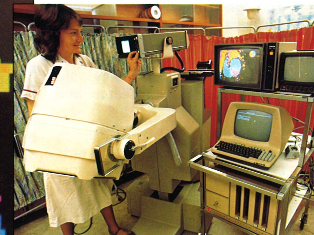
Gamma Camera/Computer system - developed in Edinburgh's Department of Medicine - used to measure patients' heart efficiency
